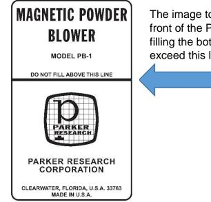
The image to the left shows the artwork printed on the front of the PB1 Bottle. Make note of the fill line when filling the bottle with powder. The powder should not exceed this line.
